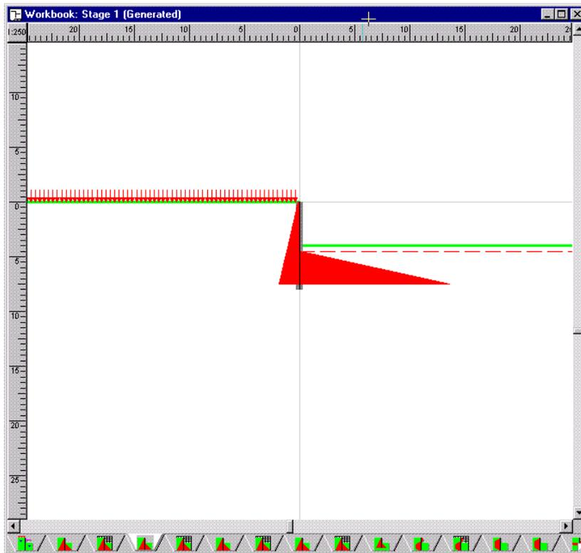
Note that the earth pressures on the excavated side of the wall do not begin at formation level – this is because BS 8002 requires a minimum unplanned excavation of 0.5m to be included in the calculations. (One of ReWaRD’s key benefits is that important details like this are automatically applied.)
